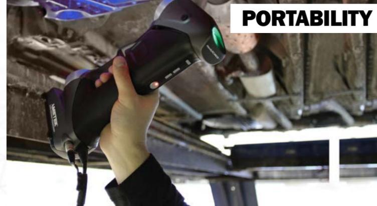
Using triangulation on optical reflectors to determine its relative position to the part, this handheld 3D scanner is a stand-alone device that does not require a tripod or any external tracking device to operate. Compact enough to fit into a small suitcase, it can be brought anywhere and used in any environmental conditions without its performance being affected.
